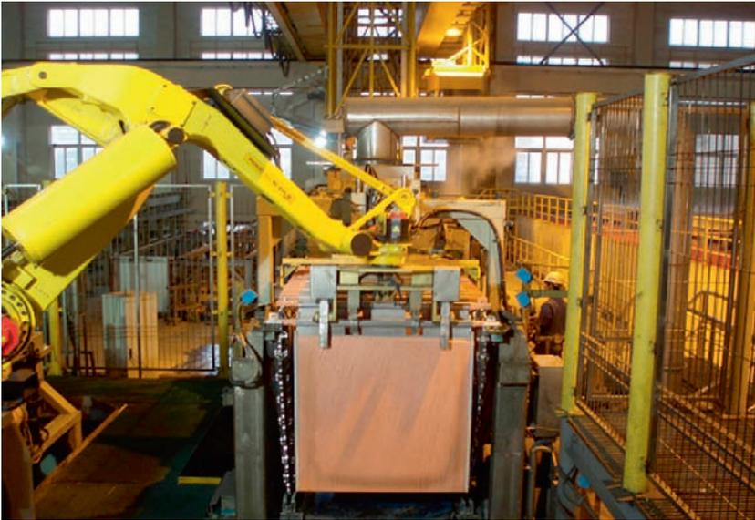
**FIGURE 14.6** Xstrata Technology robotic cathode stripping machine, manufactured by Ionic Engineering Limited, installed at an Asian copper refinery. (Courtesy of Xstrata Technologies.)
