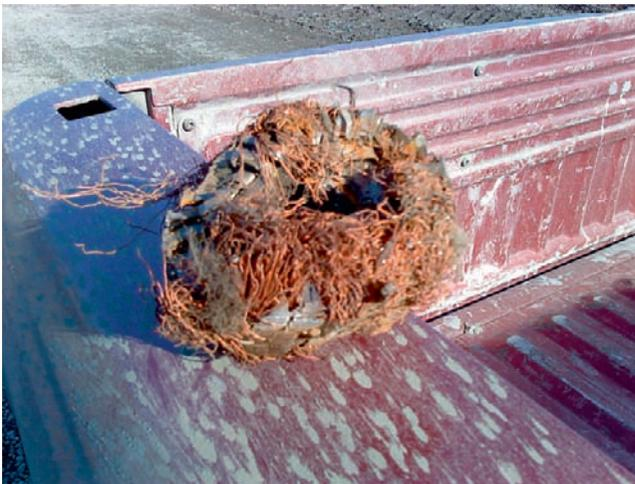
**FIGURE 18.5** *Meatballs* are created when electric motors are shredded, resulting in a commingled mix of copper wire and iron motor core. (Photo courtesy Zane Voss, Nucor, Inc.)
