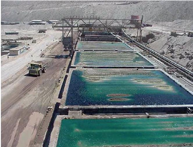
**FIGURE 15.12** Vat leaching at Mantos Blancos in Chile. Approximately 40 000 t/a Cu are produced from leaching in 12 vats. It is the only site in the world that still uses this leaching technology, although there is currently renewed interest in its application (Mackie & Trask, 2009; Schlitt & Johnston, 2010). (Courtesy of Anglo American.)
