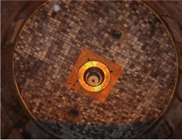
**FIGURE 10.1** New Chingola direct-to-copper flash furnace. The photo shows the top of the reaction shaft and the bottom tip of the concentrate burner. The diameter of the reaction shaft is ~6 m. Photograph by W.G. Davenport.
