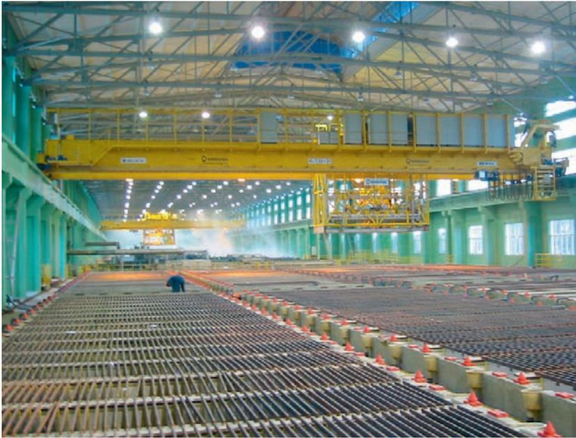
**FIGURE 14.2** A modern copper electrorefinery in China. Note the overhead crane used for moving anodes and cathodes to and from the cells. In the background, the plastic sheets covering some of the cells minimize evaporation and heat losses, thereby minimizing energy consumption. (Courtesy of Outotec.)
