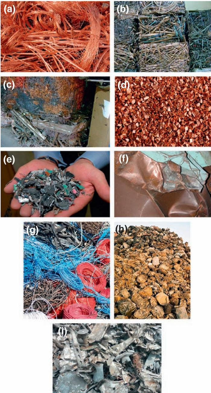
**FIGURE 18.2** Grades of copper scrap: (a) No. 1 copper wire (ISRI code Barley/Berry), (b) No. 1 heavy copper (Candy), (c) No. 2 heavy copper (Cliff), (d) Chopped copper wire (Clove/Cobra/Cocoa), (e) Upgraded shredded electronic scrap (Dallas), (f) Light copper scrap (Dream), (g) Insulated wire scrap (Druid), (h) Shredded electric motors (Shelmo), (i) Upgraded auto shredder residue (Zebra). All photographs courtesy ISRI, International, except (e) Wallach Iron & Metal, and (i) Lynx Recyclers.
