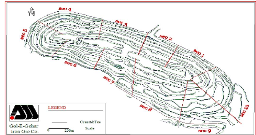
Figure 2-3: Golgohar Mine 1 Open Pit Geotechnical Domains
