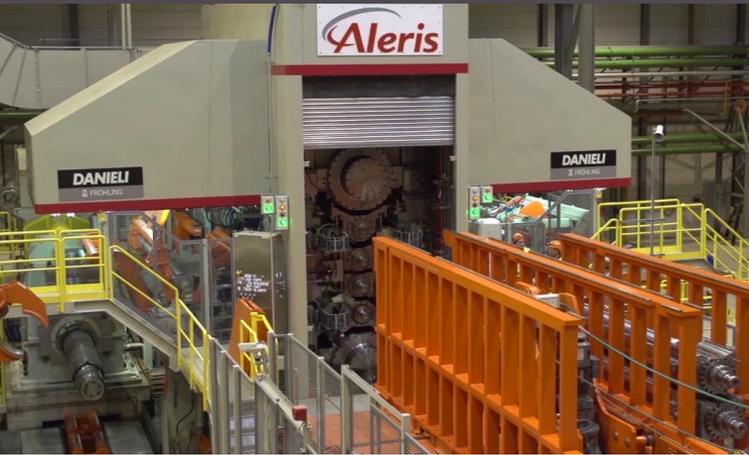
**Aluminium strip produced with the innovative Alcoa Danieli Micromill process which offers improved mechanical characteristics: see possible production of 7xxx alloys to compete with steel.**
